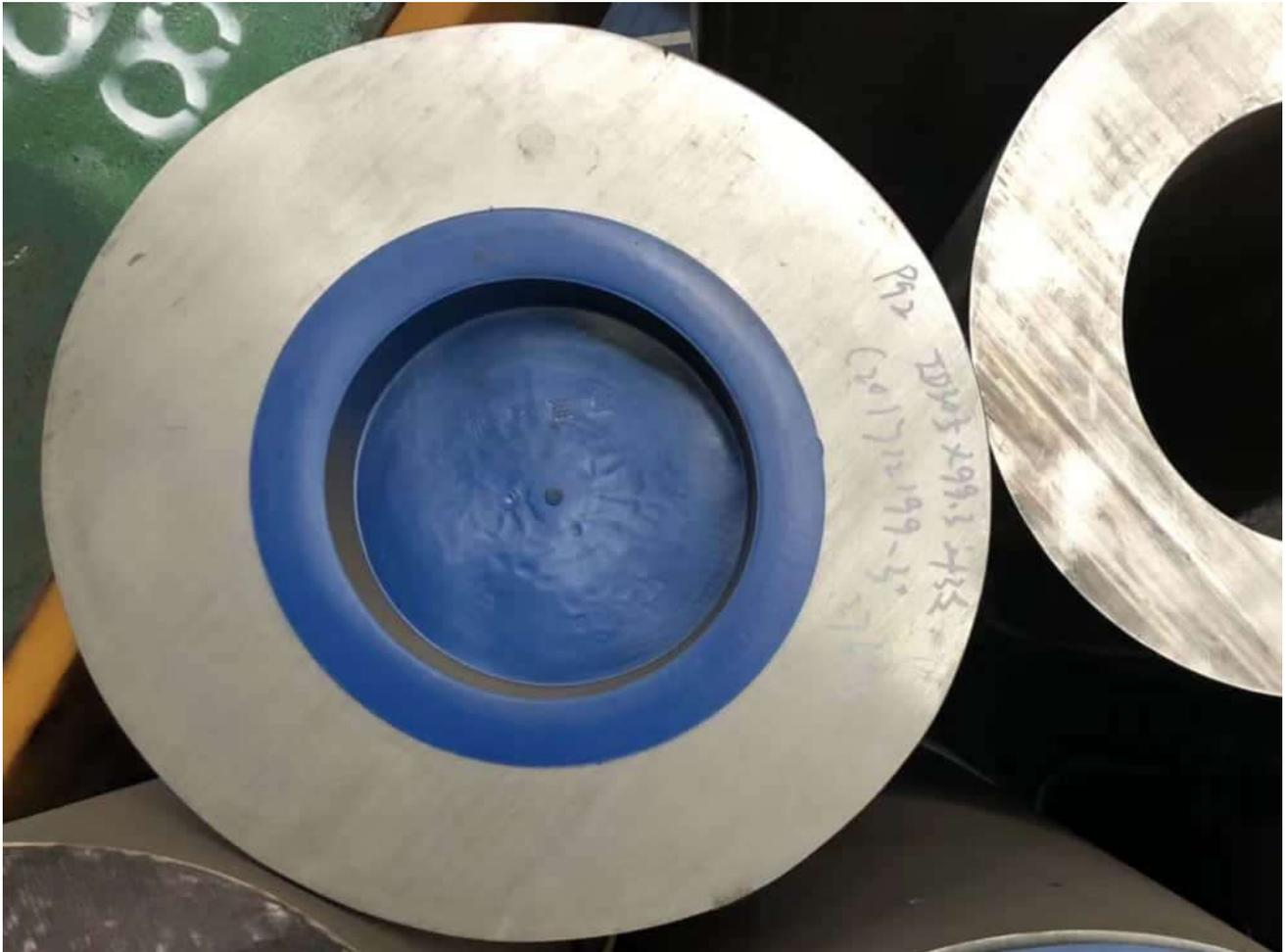
ASTM A335 P92 pipe shall be suitable for bending, flanging, and similar forming operations, and for fusion welding.
