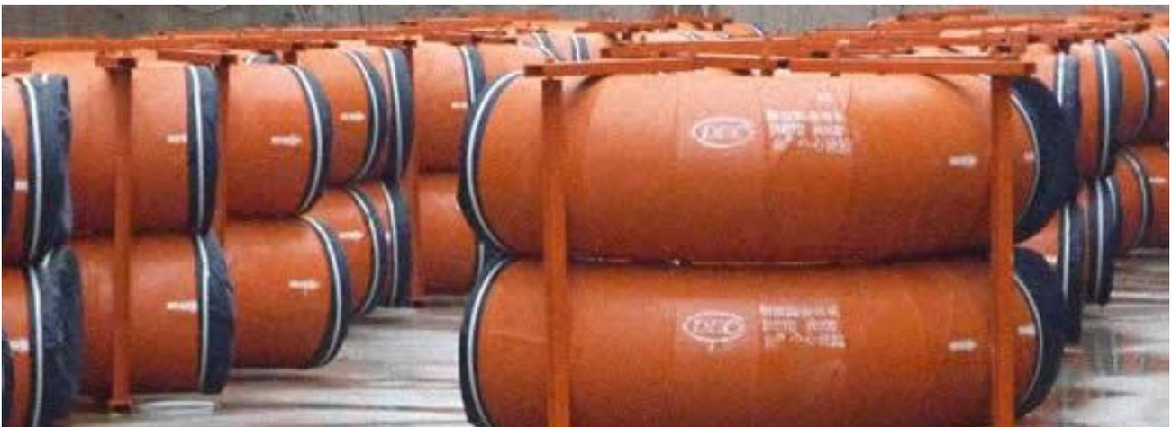
Bi-metal Clad Pipe and Bend are cast with mold vanishing vacuum suction casting cladding process.
