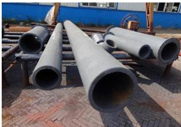
Outer of bend uses hot-bending bend and lining is cast with high-chromium cast iron. Bends and other profile sections can be clad in whole and this process has changed the traditional practice to fabricate bend and other profile sections by drawing polyline without changing flow pattern of material inside piping, greatly reducing conveyance resistance of material.
