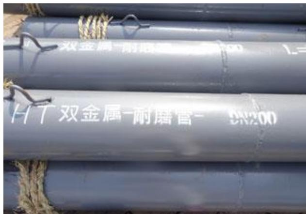
Bimetallic lined with high chrome alloy pipe High chromium alloy material by a special process of a one-time casting shape.
