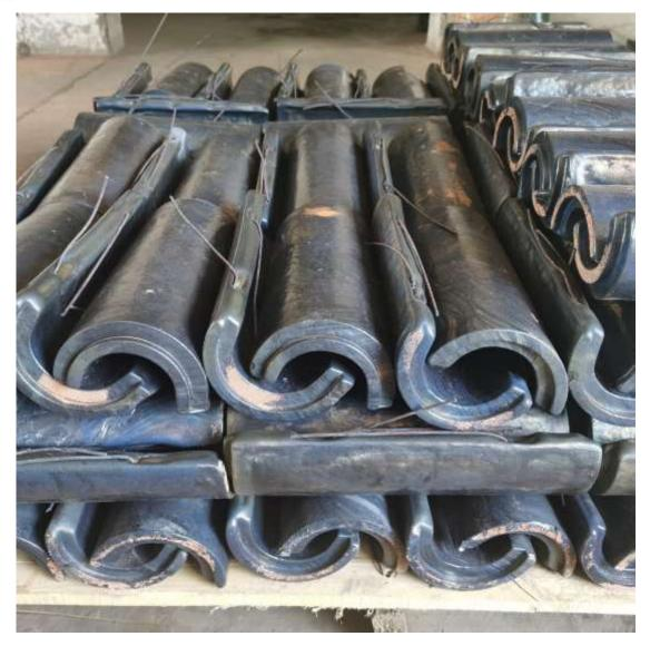
It is usually used in power station boilers. The useful life of tube shield is 3-5 years. The tube shield has a variety of material and the selection of the material shall be subject to the original design of the boiler. The tube shield is divided into straight pipe
