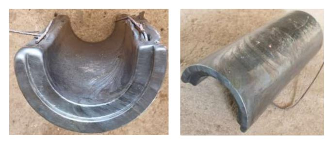
Cast basalt pipe shield is a common component of the heating part of tubes.
