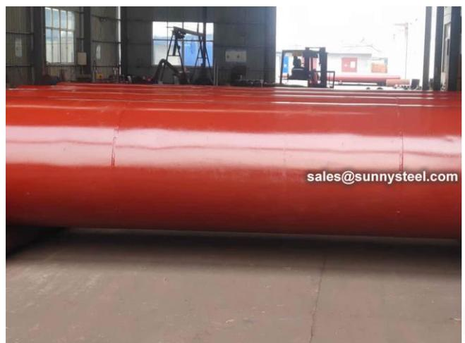
Out diameter 1020mm ceramic lined pipe
