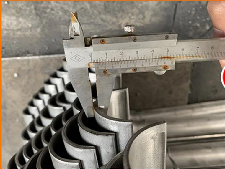
Wall thickness inspection by third party
